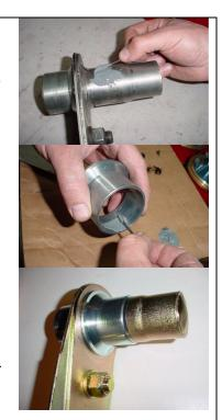
4 - Install bearings into the spring plate cover plates.
